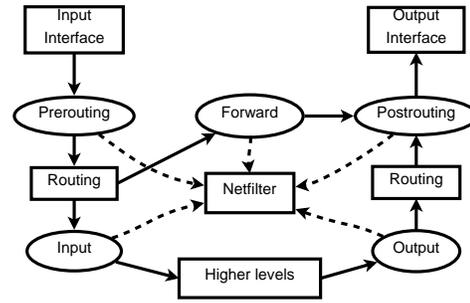
Fig. 4. The packet filter mechanism
